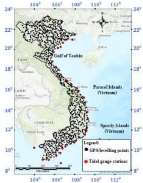
Figure 3.6. The GPS/levelling and tidal gauge station's locations in the territory of Vietnam
